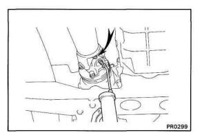
3. APPLY MP GREASE TO GREASE FITTING
