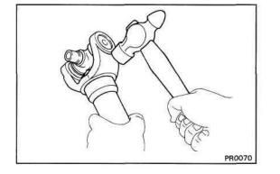
(e) Using SST, adjust both bearings so that the snap ring grooves are at maximum and equal widths.
